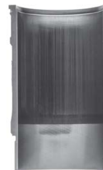
Severely Scuffed Liner
